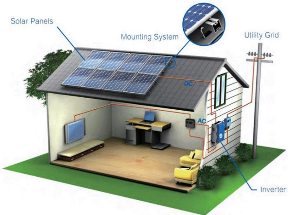
Fig.1. Rooftop Solar System
